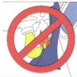
Exposed light bulbs can be a fire hazard. Ensure light bulbs, especially in the engine room, are covered by globes.
