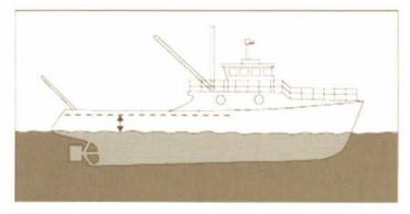
A proper freeboard is essential for stability. Freeboard is the distance between the water and the working deck of the vessel. If the deck edge goes under the water when the vessel heels, the danger of capsizing is great.
