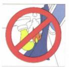
Exposed light bulbs can be a fire hazard. Ensure light bulbs, especially in the engine room, are covered by globes.
